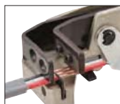
stripping inner sheath
