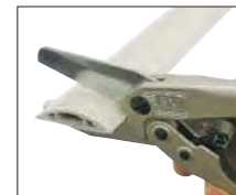
Cutting of cable protector
