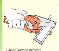
Plastic surface raceway. (up to W30mm×H10mm)
