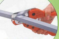
Possible to cut plastic surface raceway at any desired angle with an attachment (option) installed.
