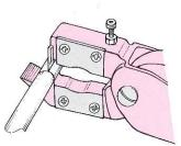
Then insert the blade into the stripped line, and remove the coating by turning the cable.
